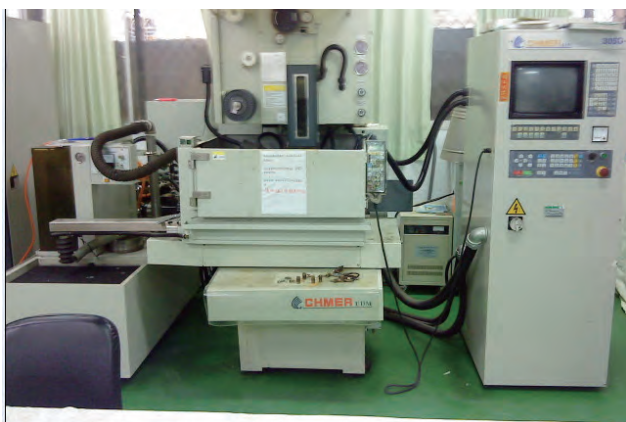
▲ Wire-cutting machine with smart manufacture
